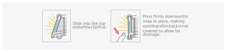
**4.** Starting with the connected end, snap the Mounting Channel into the clips (for open channel extrusion: slot on bottom rear). Be careful not to bend or kink the Light Tape® when snapping into place. Be sure that the end of extrusion or bottom rear slit (if using open channel extrusion) are not covered or sealed, especially when using UltraBond™ to mount. This allows for proper air flow and drainage.
